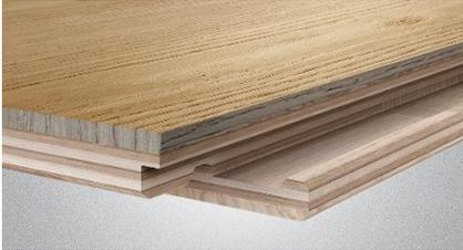
Floors with a total thickness of 13.3 mm and 10,5 mm, with a 2.7 mm-thick renovatable wood layer. Such a thickness makes it possible to renovate the floor two times. The floors are installed in the 2LOC system. They perform well in interiors fitted with underfloor heating. They are finished with 7 coatings of varnish. The structure is made of spruce wood, which is characterised by high resistance to room humidity and temperature fluctuations throughout the year.
