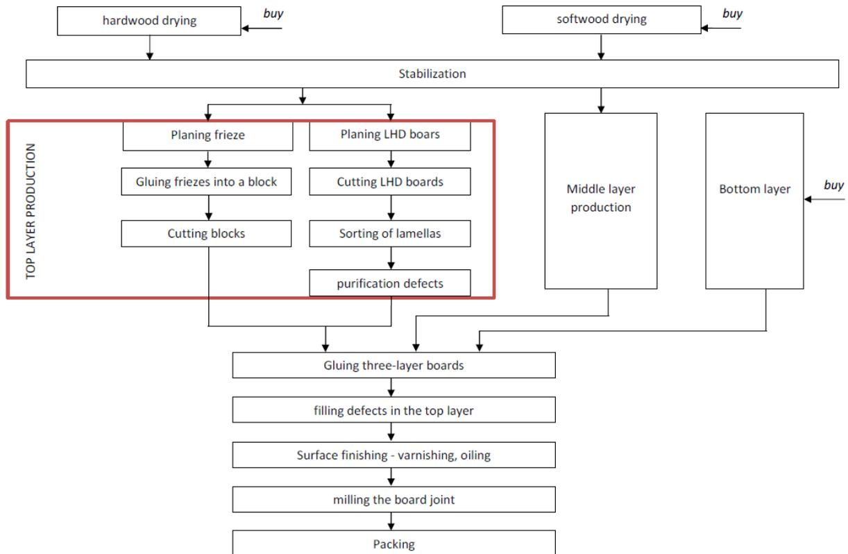
Fig. 3. A scheme of the 3-layer wooden floorboard production by Baltic Wood S.A. factory (Jasło, Poland)
