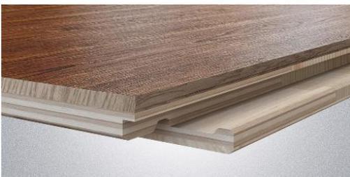
Floors with a total thickness of 14 mm and 21,3 mm, with a 3.5 mm-thick renovatable layer, which makes it possible to renovate the floor up to 3 times. They are installed in the 5G, T&G and 2LOC systems (14 mm) and T&G system (21,3 mm). The structure is made of spruce wood, which is characterised by high resistance to room humidity and temperature fluctuations throughout the year. The boards are finished with 7 coatings of varnish or 2 coatings of oil.
