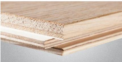
Floors of a total thickness of 14.6 mm. Thanks to the renovatable layer of as many as 6.6 mm, this type of flooring may be renovated up to 9 times. The structure is made of spruce wood, which is characterised by high resistance to room humidity and temperature fluctuations throughout the year. The boards are finished with 7 coatings of varnish or 2 coatings of oil. Glued down to the subfloor, in the T&G installation system.
