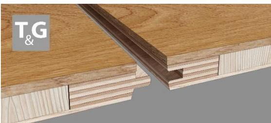
A traditional adhesive-based tongue-and-groove joint. The joint becomes durable after a dedicated engineering adhesive has been applied and has set. The adhesive is applied on the long and short sides of the board, and along the whole of the groove. The durability of the joint will be conditional upon the parameters of the applied adhesive.
