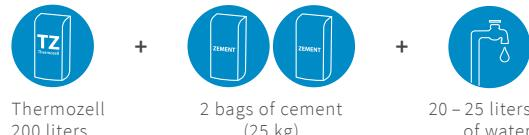
The mixing process with the addition of cement and water takes place at the construction site. Different amounts of cement are added to produce the product types pro 400, 250 and 160 speed with the respective properties.
