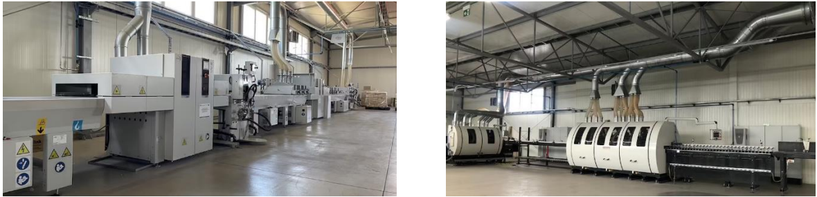
Fig. 1 Production line for UV oiling and varnishing (left) and a line for profiling floors (right) of Podłogi Sp. z o.o. production plant located in Łańcut (Poland).
